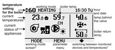
\*CAUTION - Temperature of the stoker is displayed on the "manual mode" screen of the stoker and blower - press [MODE], and then [MANUAL MODE].
