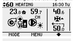
While adding coal into the hopper press [MODE] and then press [STOP] on the [WORKING MODE] screen.
